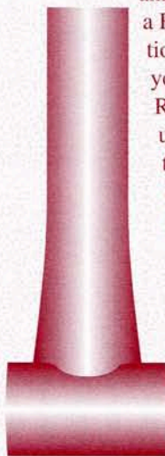
Seat tube and down tube are ovalized at the bottom bracket
